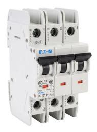
Eaton miniature circuit breaker, current-limiting, 13A, 240 VAC / 96 VDC, 3-pole, D curve, thermal magnetic, 14kA @ 240 VAC interrupting rating, 35mm DIN rail mount.
