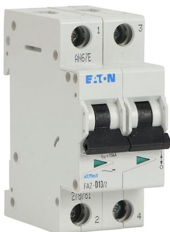
Eaton miniature supplementary protector, 13A, 480Y / 277 VAC / 96 VDC, 2-pole, D curve, thermal magnetic, 5kA @ 480Y/277 VAC interrupting rating, 35mm DIN rail mount.
