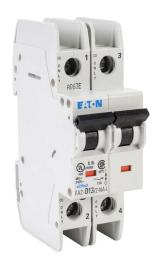
Eaton miniature circuit breaker, current-limiting, 13A, 240 VAC / 96 VDC, 2-pole, D curve, thermal magnetic, 14kA @ 240 VAC interrupting rating, 35mm DIN rail mount.
