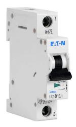
Eaton miniature supplementary protector, 13A, 277 VAC / 48 VDC, 1-pole, D curve, thermal magnetic, 5kA @ 277 VAC interrupting rating, 35mm DIN rail mount.
