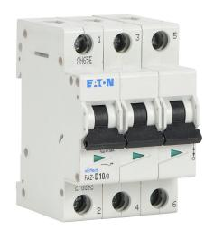
Eaton miniature supplementary protector, 10A, 480Y / 277 VAC / 96 VDC, 3-pole, D curve, thermal magnetic, 5kA @ 480Y/277 VAC interrupting rating, 35mm DIN rail mount.
