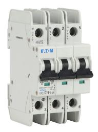
Eaton miniature circuit breaker, current-limiting, 10A, 480Y / 277 VAC / 96 VDC, 3-pole, D curve, thermal magnetic, 10kA @ 480Y/277 VAC interrupting rating, 35mm DIN rail mount.
