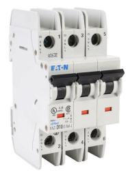
Eaton miniature circuit breaker, current-limiting, 10A, 240 VAC / 96 VDC, 3-pole, D curve, thermal magnetic, 10kA @ 240 VAC interrupting rating, 35mm DIN rail mount.
