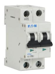
Eaton miniature supplementary protector, 10A, 480Y / 277 VAC / 96 VDC, 2-pole, D curve, thermal magnetic, 5kA @ 480Y/277 VAC interrupting rating, 35mm DIN rail mount.
