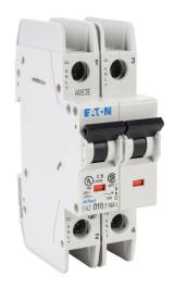
Eaton miniature circuit breaker, current-limiting, 10A, 240 VAC / 96 VDC, 2-pole, D curve, thermal magnetic, 10kA @ 240 VAC interrupting rating, 35mm DIN rail mount.
