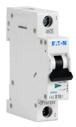
Eaton miniature supplementary protector, 10A, 277 VAC / 48 VDC, 1-pole, D curve, thermal magnetic, 5kA @ 277 VAC interrupting rating, 35mm DIN rail mount.
