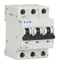
Eaton miniature supplementary protector, 1A, 480Y / 277 VAC / 96 VDC, 3-pole, D curve, thermal magnetic, 5kA @ 480Y/277 VAC interrupting rating, 35mm DIN rail mount.
