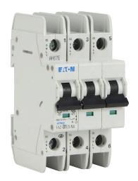
Eaton miniature circuit breaker, current-limiting, 1A, 480Y / 277 VAC / 96 VDC, 3-pole, D curve, thermal magnetic, 10kA @ 480Y/277 VAC interrupting rating, 35mm DIN rail mount.
