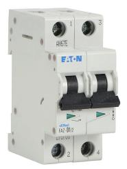
Eaton miniature supplementary protector, 1A, 480Y / 277 VAC / 96 VDC, 2-pole, D curve, thermal magnetic, 5kA @ 480Y/277 VAC interrupting rating, 35mm DIN rail mount.
