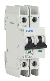
Eaton miniature circuit breaker, current-limiting, 1A, 480Y / 277 VAC / 96 VDC, 2-pole, D curve, thermal magnetic, 10kA @ 480Y/277 VAC interrupting rating, 35mm DIN rail mount.
