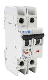
Eaton miniature circuit breaker, current-limiting, 1A, 240 VAC / 96 VDC, 2-pole, D curve, thermal magnetic, 10kA @ 240 VAC interrupting rating, 35mm DIN rail mount.
