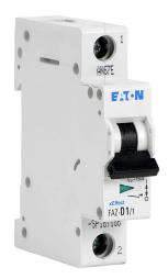
Eaton miniature supplementary protector, 1A, 277 VAC / 48 VDC, 1-pole, D curve, thermal magnetic, 5kA @ 277 VAC interrupting rating, 35mm DIN rail mount.
