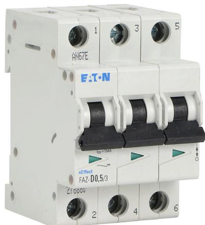
Eaton miniature supplementary protector, 0.5A, 480Y / 277 VAC / 96 VDC, 3-pole, D curve, thermal magnetic, 5kA @ 480Y/277 VAC interrupting rating, 35mm DIN rail mount.
