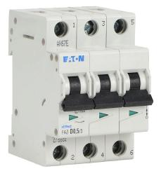
Eaton miniature supplementary protector, 0.5A, 480Y / 277 VAC / 96 VDC, 3-pole, D curve, thermal magnetic, 5kA @ 480Y/277 VAC interrupting rating, 35mm DIN rail mount.
