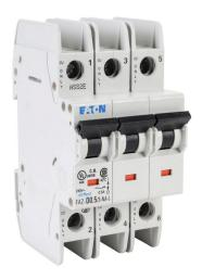
Eaton miniature circuit breaker, current-limiting, 0.5A, 240 VAC / 96 VDC, 3-pole, D curve, thermal magnetic, 10kA @ 240 VAC interrupting rating, 35mm DIN rail mount.
