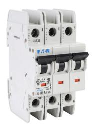
Eaton miniature circuit breaker, current-limiting, 0.5A, 240 VAC / 96 VDC, 3-pole, D curve, thermal magnetic, 10kA @ 240 VAC interrupting rating, 35mm DIN rail mount.
