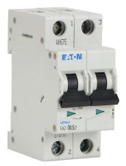
Eaton miniature supplementary protector, 0.5A, 480Y / 277 VAC / 96 VDC, 2-pole, D curve, thermal magnetic, 5kA @ 480Y/277 VAC interrupting rating, 35mm DIN rail mount.
