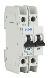
Eaton miniature circuit breaker, current-limiting, 0.5A, 480Y / 277 VAC / 96 VDC, 2-pole, D curve, thermal magnetic, 10kA @ 480Y/277 VAC interrupting rating, 35mm DIN rail mount.
