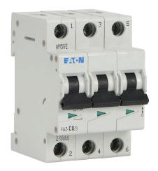
Eaton miniature supplementary protector, 8A, 480Y / 277 VAC / 96 VDC, 3-pole, C curve, thermal magnetic, 10kA @ 480Y/277 VAC interrupting rating, 35mm DIN rail mount.
