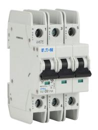
Eaton miniature circuit breaker, current-limiting, 8A, 480Y / 277 VAC / 96 VDC, 3-pole, C curve, thermal magnetic, 10kA @ 480Y/277 VAC interrupting rating, 35mm DIN rail mount.
