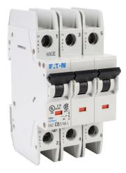
Eaton miniature circuit breaker, current-limiting, 8A, 240 VAC / 96 VDC, 3-pole, C curve, thermal magnetic, 10kA @ 240 VAC interrupting rating, 35mm DIN rail mount.
