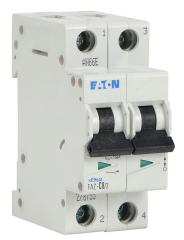
Eaton miniature supplementary protector, 8A, 480Y / 277 VAC / 96 VDC, 2-pole, C curve, thermal magnetic, 10kA @ 480Y/277 VAC interrupting rating, 35mm DIN rail mount.
