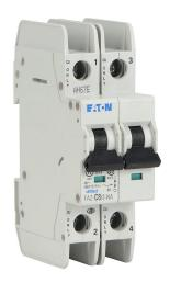
Eaton miniature circuit breaker, current-limiting, 8A, 480Y / 277 VAC / 96 VDC, 2-pole, C curve, thermal magnetic, 10kA @ 480Y/277 VAC interrupting rating, 35mm DIN rail mount.
