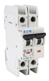
Eaton miniature circuit breaker, current-limiting, 8A, 240 VAC / 96 VDC, 2-pole, C curve, thermal magnetic, 10kA @ 240 VAC interrupting rating, 35mm DIN rail mount.
