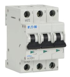
Eaton miniature supplementary protector, 7A, 480Y / 277 VAC / 96 VDC, 3-pole, C curve, thermal magnetic, 10kA @ 480Y/277 VAC interrupting rating, 35mm DIN rail mount.
