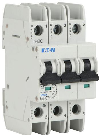
Eaton miniature circuit breaker, current-limiting, 7A, 480Y / 277 VAC / 96 VDC, 3-pole, C curve, thermal magnetic, 10kA @ 480Y/277 VAC interrupting rating, 35mm DIN rail mount.
