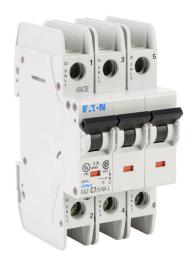
Eaton miniature circuit breaker, current-limiting, 7A, 240 VAC / 96 VDC, 3-pole, C curve, thermal magnetic, 10kA @ 240 VAC interrupting rating, 35mm DIN rail mount.
