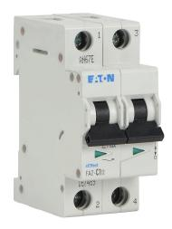
Eaton miniature supplementary protector, 7A, 480Y / 277 VAC / 96 VDC, 2-pole, C curve, thermal magnetic, 10kA @ 480Y/277 VAC interrupting rating, 35mm DIN rail mount.
