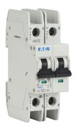
Eaton miniature circuit breaker, current-limiting, 7A, 480Y / 277 VAC / 96 VDC, 2-pole, C curve, thermal magnetic, 10kA @ 480Y/277 VAC interrupting rating, 35mm DIN rail mount.
