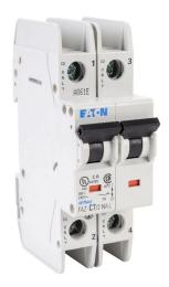
Eaton miniature circuit breaker, current-limiting, 7A, 240 VAC / 96 VDC, 2-pole, C curve, thermal magnetic, 10kA @ 240 VAC interrupting rating, 35mm DIN rail mount.
