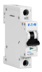
Eaton miniature supplementary protector, 7A, 277 VAC / 48 VDC, 1-pole, C curve, thermal magnetic, 10kA @ 277 VAC interrupting rating, 35mm DIN rail mount.
