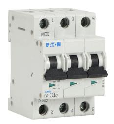
Eaton miniature supplementary protector, 63A, 480Y / 277 VAC / 96 VDC, 3-pole, C curve, thermal magnetic, 5kA @ 480Y/277 VAC interrupting rating, 35mm DIN rail mount.
