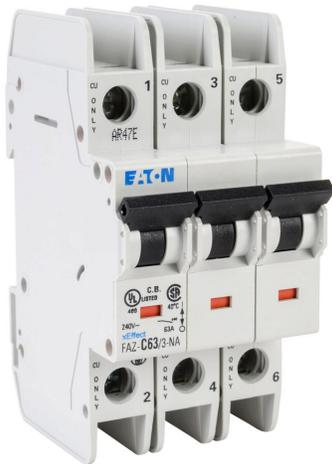
Eaton miniature circuit breaker, current-limiting, 63A, 240 VAC / 96 VDC, 3-pole, C curve, thermal magnetic, 10kA @ 240 VAC interrupting rating, 35mm DIN rail mount.
