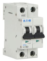
Eaton miniature supplementary protector, 63A, 480Y / 277 VAC / 96 VDC, 2-pole, C curve, thermal magnetic, 5kA @ 480Y/277 VAC interrupting rating, 35mm DIN rail mount.
