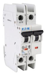
Eaton miniature circuit breaker, current-limiting, 63A, 240 VAC / 96 VDC, 2-pole, C curve, thermal magnetic, 10kA @ 240 VAC interrupting rating, 35mm DIN rail mount.
