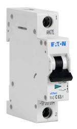
Eaton miniature supplementary protector, 63A, 277 VAC / 48 VDC, 1-pole, C curve, thermal magnetic, 5kA @ 277 VAC interrupting rating, 35mm DIN rail mount.
