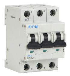
Eaton miniature supplementary protector, 6A, 480Y / 277 VAC / 96 VDC, 3-pole, C curve, thermal magnetic, 10kA @ 480Y/277 VAC interrupting rating, 35mm DIN rail mount.
