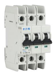
Eaton miniature circuit breaker, current-limiting, 6A, 480Y / 277 VAC / 96 VDC, 3-pole, C curve, thermal magnetic, 10kA @ 480Y/277 VAC interrupting rating, 35mm DIN rail mount.
