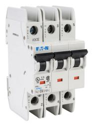
Eaton miniature circuit breaker, current-limiting, 6A, 240 VAC / 96 VDC, 3-pole, C curve, thermal magnetic, 10kA @ 240 VAC interrupting rating, 35mm DIN rail mount.
