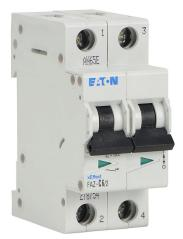
Eaton miniature supplementary protector, 6A, 480Y / 277 VAC / 96 VDC, 2-pole, C curve, thermal magnetic, 10kA @ 480Y/277 VAC interrupting rating, 35mm DIN rail mount.
