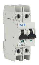
Eaton miniature circuit breaker, current-limiting, 6A, 480Y / 277 VAC / 96 VDC, 2-pole, C curve, thermal magnetic, 10kA @ 480Y/277 VAC interrupting rating, 35mm DIN rail mount.
