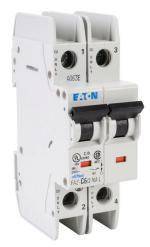
Eaton miniature circuit breaker, current-limiting, 6A, 240 VAC / 96 VDC, 2-pole, C curve, thermal magnetic, 10kA @ 240 VAC interrupting rating, 35mm DIN rail mount.
