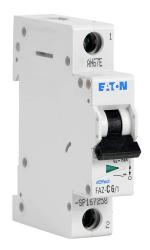
Eaton miniature supplementary protector, 6A, 277 VAC / 48 VDC, 1-pole, C curve, thermal magnetic, 10kA @ 277 VAC interrupting rating, 35mm DIN rail mount.
