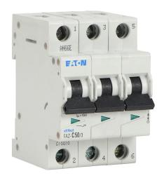
Eaton miniature supplementary protector, 50A, 480Y / 277 VAC / 96 VDC, 3-pole, C curve, thermal magnetic, 5kA @ 480Y/277 VAC interrupting rating, 35mm DIN rail mount.
