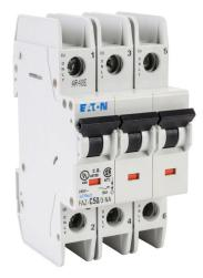
Eaton miniature circuit breaker, current-limiting, 50A, 240 VAC / 96 VDC, 3-pole, C curve, thermal magnetic, 10kA @ 240 VAC interrupting rating, 35mm DIN rail mount.
