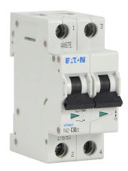
Eaton miniature supplementary protector, 50A, 480Y / 277 VAC / 96 VDC, 2-pole, C curve, thermal magnetic, 5kA @ 480Y/277 VAC interrupting rating, 35mm DIN rail mount.
