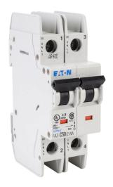
Eaton miniature circuit breaker, current-limiting, 50A, 240 VAC / 96 VDC, 2-pole, C curve, thermal magnetic, 10kA @ 240 VAC interrupting rating, 35mm DIN rail mount.
