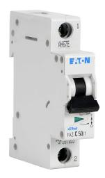
Eaton miniature supplementary protector, 50A, 277 VAC / 48 VDC, 1-pole, C curve, thermal magnetic, 5kA @ 277 VAC interrupting rating, 35mm DIN rail mount.
